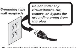
Power supply cord with 3-prong grounding plug
